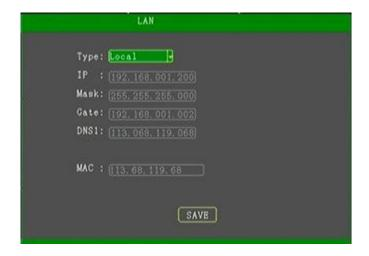
Type: way of connection incl. Local/WIFI/Peripheral(external way).
