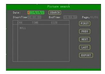
To check pictures which are saved into disk based on certain parameter setting. The picture can also be "exported" to an external u-disk.
