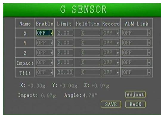
G-Sensor alarm is detected by changes from x, y and z axis. For first time of use, "Adjust" is required.
